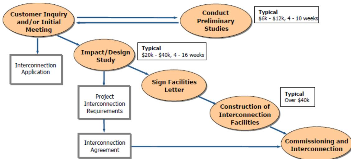
**Figure 4-3: Example of interconnection process for generators without transmission impact**
