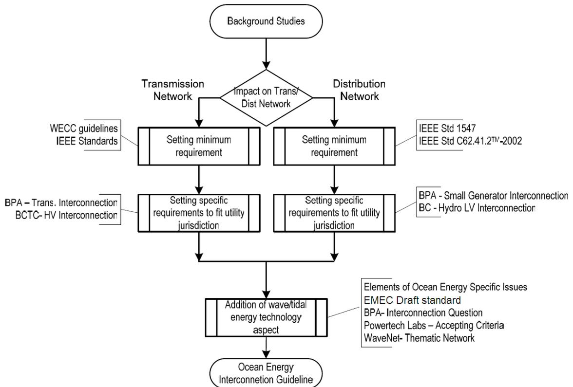
**Figure 5-1: Example of a flow-chart for ocean energy interconnection guideline development for west coasts of North America**
