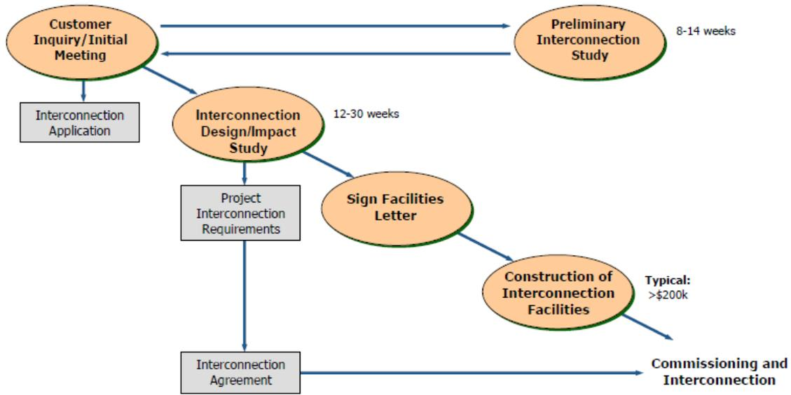
**Figure 4-2: Example of interconnection process for generators with transmission impact**
