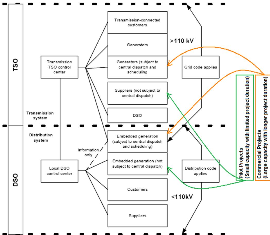
Figure 4-1: Distribution and transmission system operators' jurisdictions and project scope [9]
